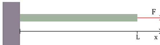
Figure 3.2.: A bar of length L , with uniform cross section A and constant Young's modulus E . No volume force or traction is present.
